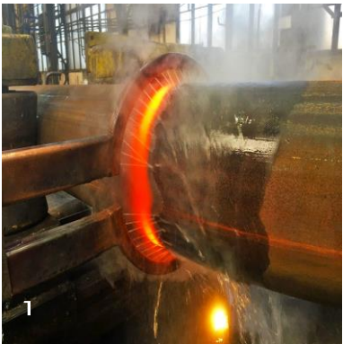
1. Bending with induction heating 2. Tube bends 3. Tube bends 4. Cold pipe bending
